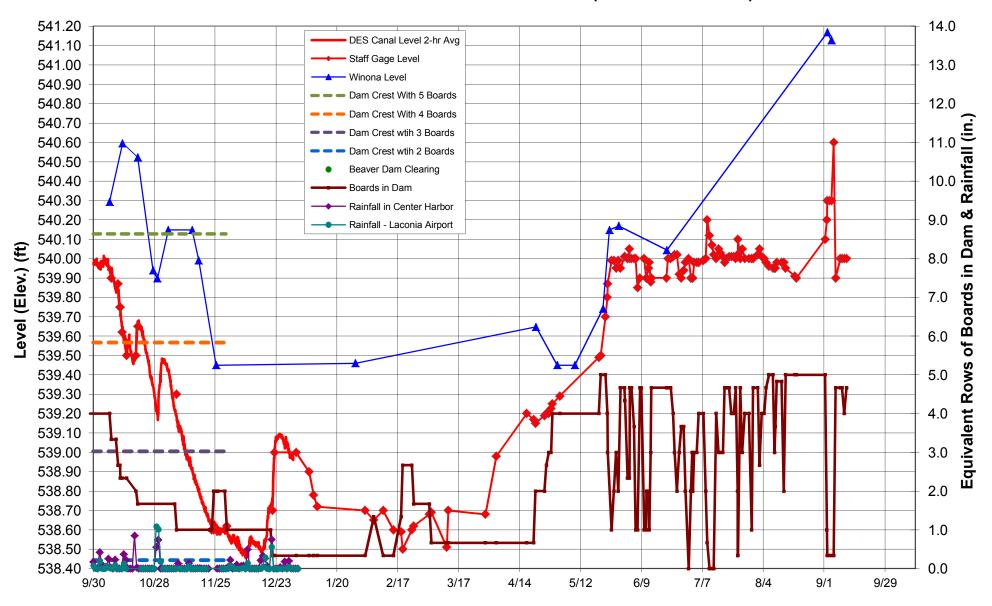
Winona data measured by volunteers at the Winona Bridge. Canal level and the number of boards in the dam and canal levels from 1/1/2013 per The Inns and Spa at Mill Falls.
