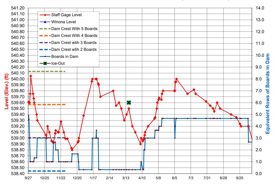
Winona data measured by volunteers at the Winona Bridge. Canal level and the number of boards in the dam and canal levels from 1/1/2013 per The Inns and Spa at Mill Falls.
